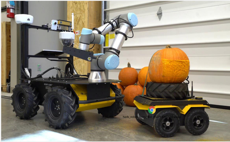
HUSKY (a medium sized robotic development platform by ClearPathRobotics)
