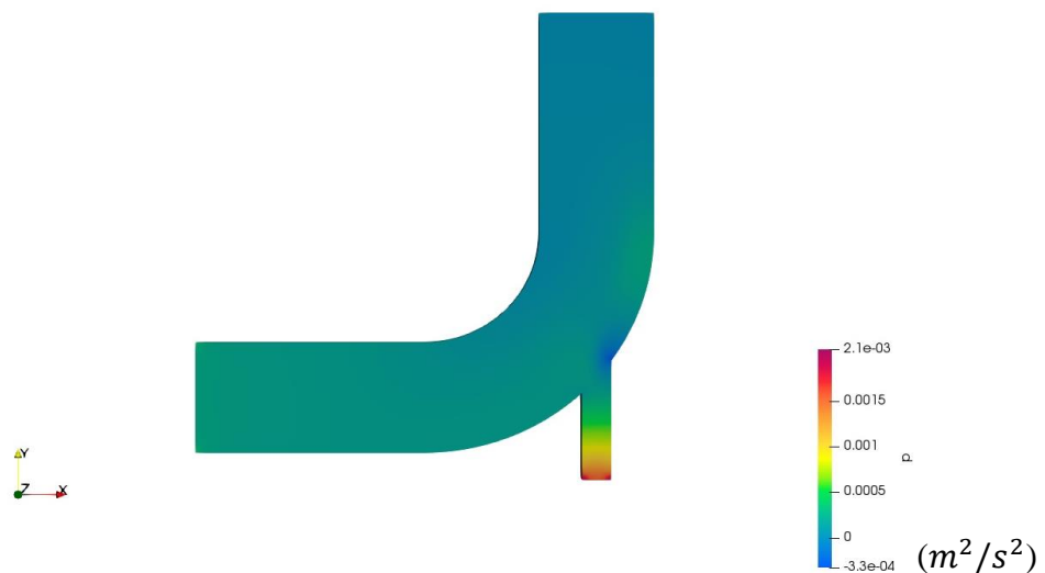
Fig. 4: Kinematic pressure distributions in the elbow obtained using modified solver in OpenFOAM at time (t) = 125 s
