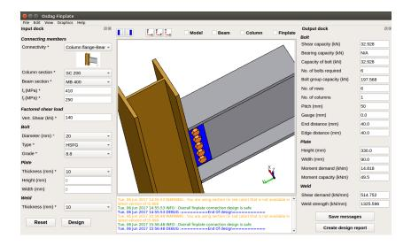
• A text window for message display, that also suggests necessary changes if a trial design is found unsafe.
