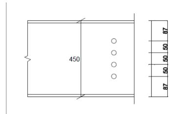
Try a cleat angle of 110x110x16. Take Fe 410 grade steel  $(f_u = 410 \text{ Mpa } \& f_y = 250 \text{ Mpa})$ .
