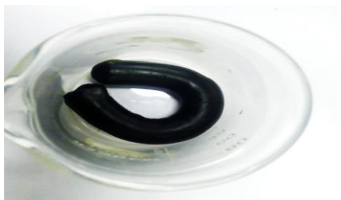
Figure 3.10 Fixing of temporary shape
